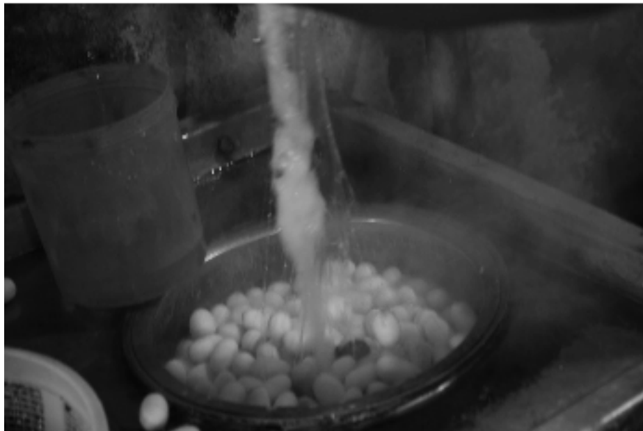
Figure 9: The boiling/cooking stage in the silk reeling process
