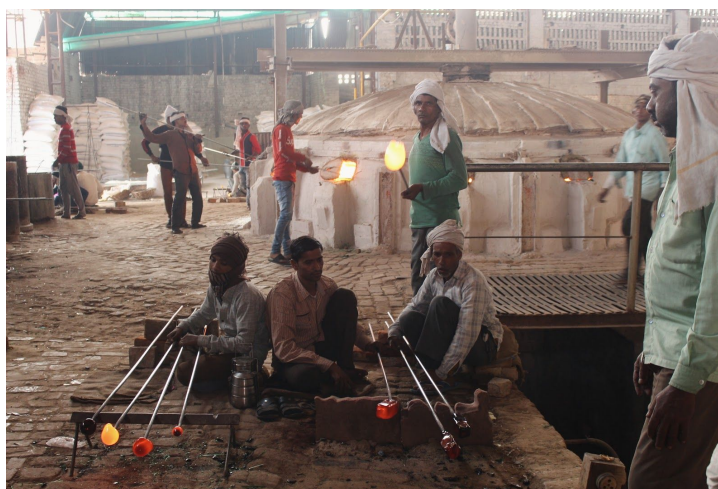
Primary shaping of the glass
