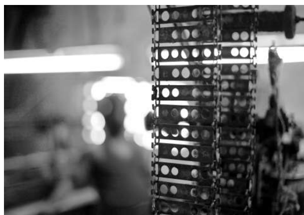
Image 18: The design card that sets patterns on the power loom
